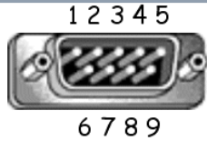
RS-232 Pin-out DB9 Male DTE
